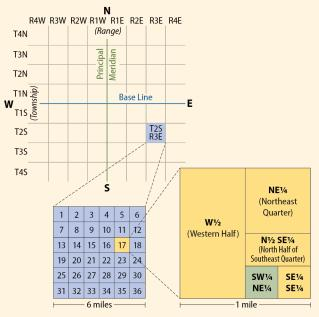
**Figure S-2.** Township (blue), section (yellow), and subsections in a U.S. Public Land Survey System grid system. This parcel (green) may be read as: Southwest quarter of the southeast quarter of Section 17, Township 2 South, Range 3 East, Mount Diablo Meridian.
