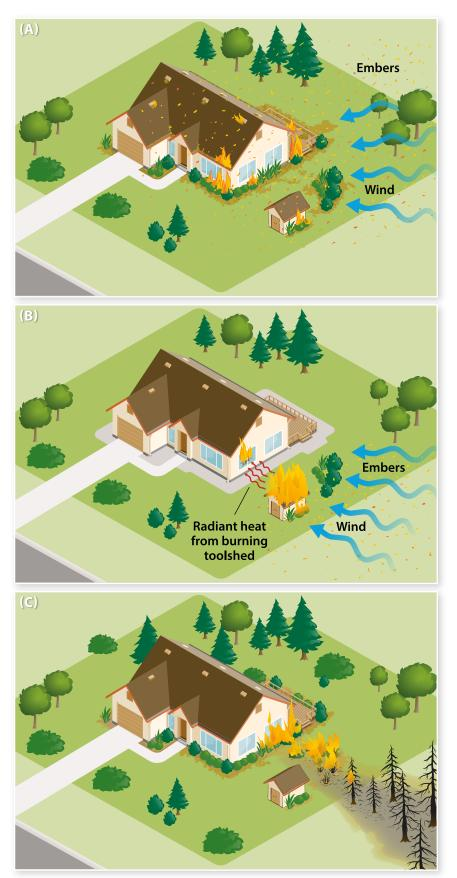
**Figure 1.** Incorporating fire safe concepts requires preparing for three different types of fire exposures—embers (A), radiant heat (B), and direct flame contact (C).
