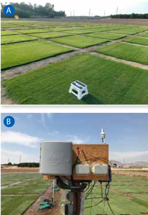
Figure 2. A turfgrass irrigation research trial at UC Riverside Agricultural Experiment Station (A), where irrigation applications are autonomously regulated by a weather-based smart irrigation controller (B). Photos: http://www.ucrwater.com .
