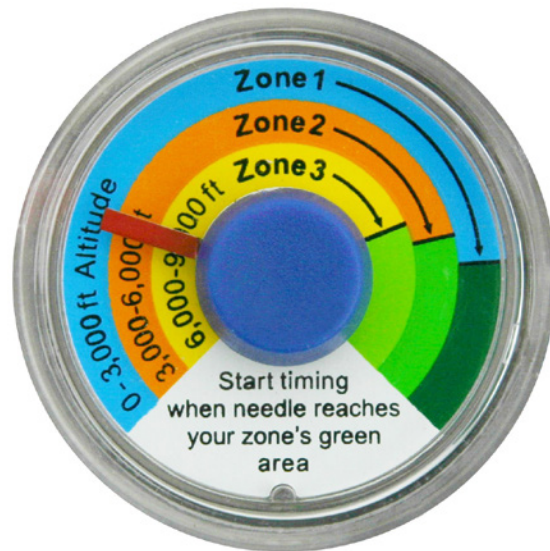
Figure 3. Victorio canner's built-in temperature gauge. Photo: Courtesy of Victorio.
