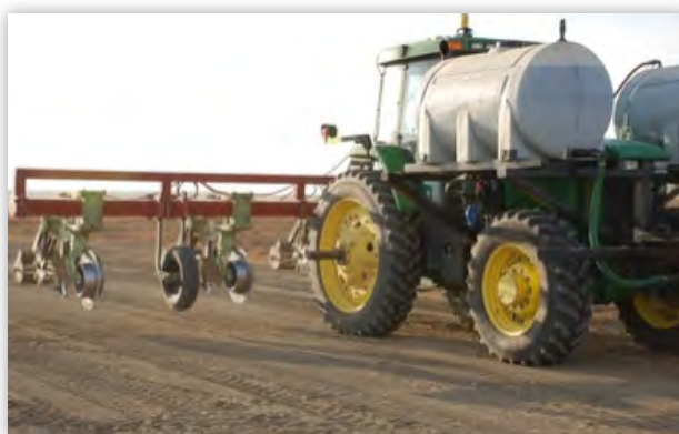
Figure 10. Close-up view of modified Orthman 1tRIPr strip-till row units at Sano Farms, showing the residue-cutting wheel and coupler, subsoiling shank, wavy coulters, and clod-busting rolling baskets.
