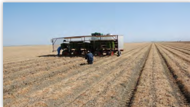
Figure 12. A conventional five-row tomato transplanter used at Sano Farms, 2009.
