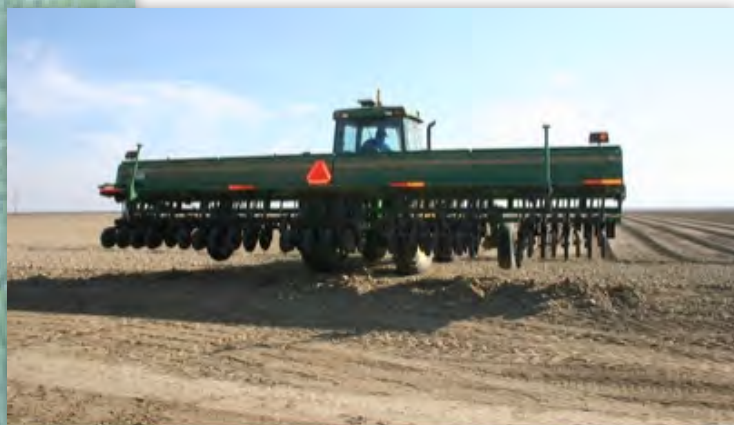
Figure 1. A 25-foot Great Plains drill is used to seed winter small grain cover crops at Sano Farms in Firebaugh, California. The modified drill plants seed across the bed top without putting any seed in the furrow.
