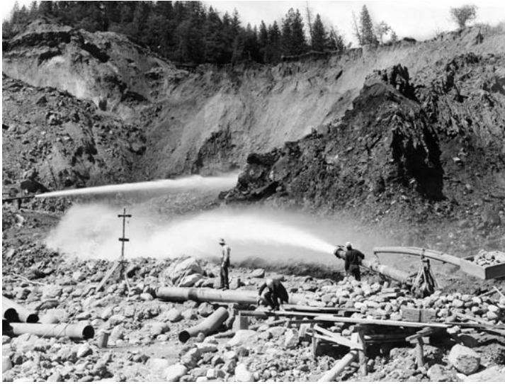
Figure 2. Hydraulic mining, 1860–1870, Trinity County. Streams were diverted through flumes, ditches, and pipes to monitors (nozzles) to wash gold-bearing gravels into sluice boxes for separation of the gold. Source: Eastman's Originals Collection Group 117, Special Collections, University of California Library, Davis, reprinted with permission.
