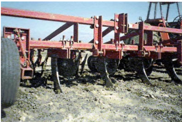
Figure 3. Close-up view of Sundance minimum-tillage bed-conditioning implement used in the Salinas Valley.
