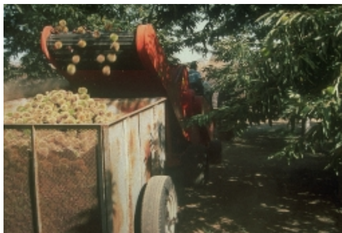
Figure 15. A conveyor belt from a pick-up machine loads chestnuts into a bin.
