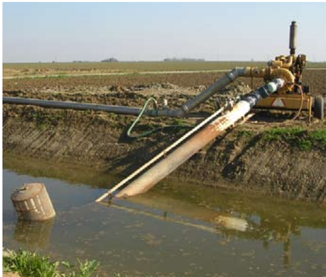
Figure 6. A rotary pump intake screen and diesel engine used for tailwater return. Photo: Lawrence J. Schwankl.
