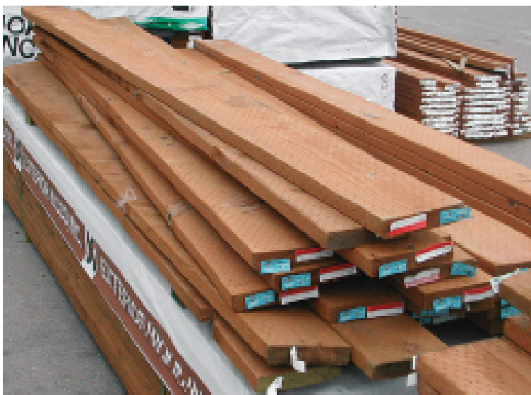
Figure 4. CCA-treated lumber can contain a brown dye to change the color from the "natural" light green color.
